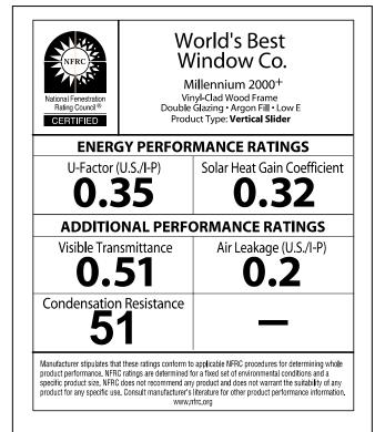
Look for the NFRC Label! The 2 most important values to look for are: U-factor & Solar Heat Gain Coefficient (SHGC)
