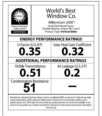
Look for the NFRC Label! The 2 most important values to look for are: U-factor & Solar Heat Gain Coefficient (SHGC)
